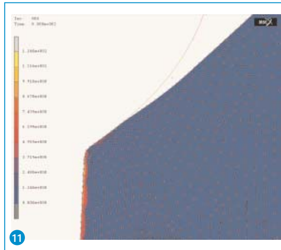
Fig. 11 Deformed mesh (pad) + contact body (plate): scalar plot of contact normal force
